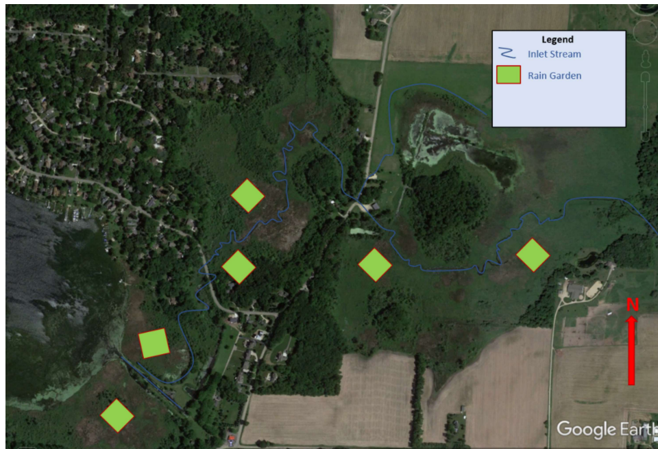
Figure 4. Map showing the inlet stream to Lake Ripley and where rain gardens will be implemented along the stream.
